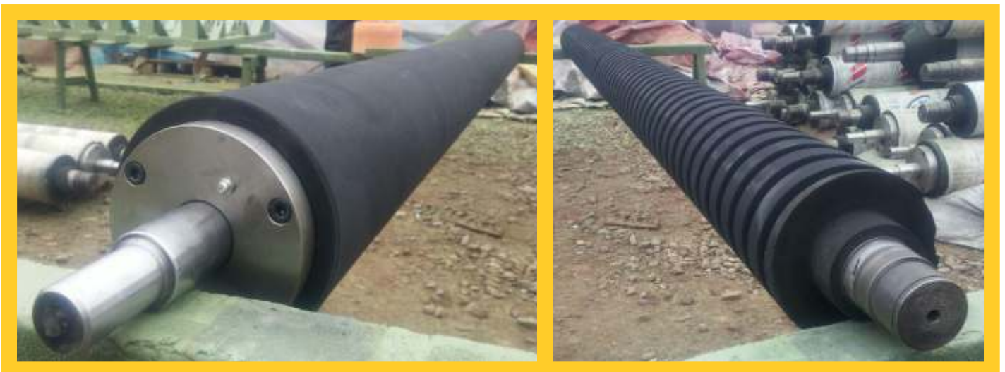
pulley with spiral veneer
